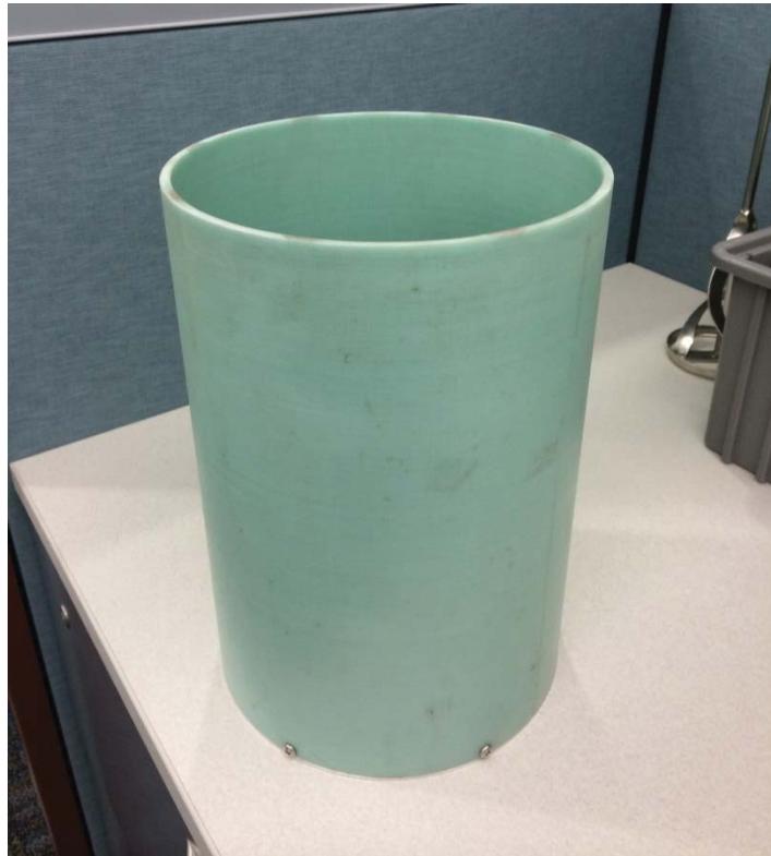
Figure 2.5 — 8" G10 specimen holder
