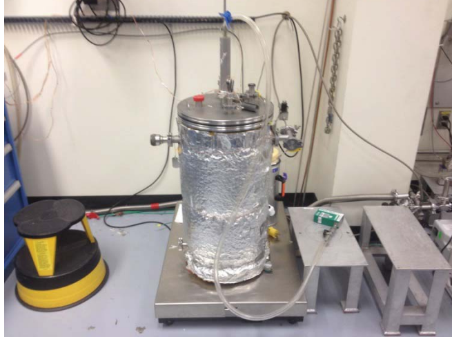
Figure 1.2 — Similar cryostat vacuum chamber used for CTL testing operation s1
