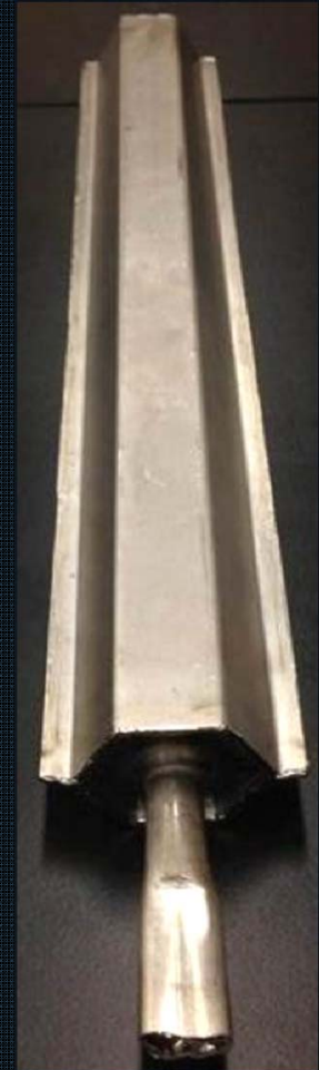
61 channel near full scale HIP can: filled and closed out
