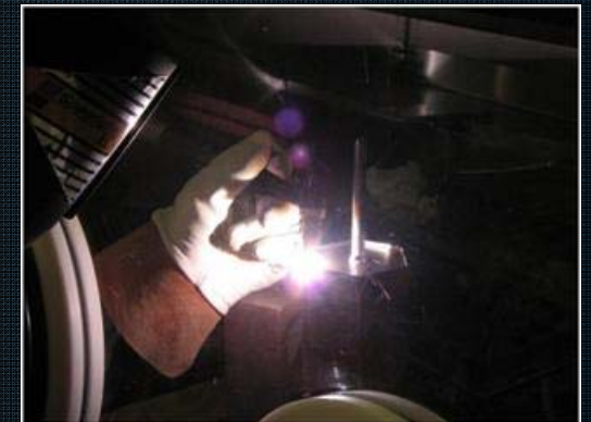
Weld in a argon glove box
