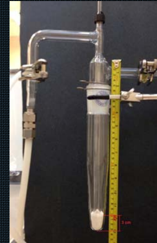
Inverted Reactor Prototype (tapered)
