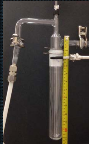
Inverted Reactor Prototype (straight)
