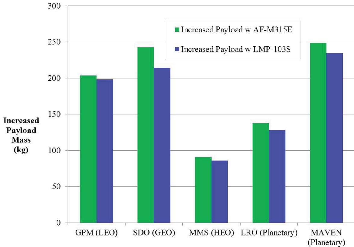
Figure 5 Additional payload mass for the same initial wet mass and delta V.
