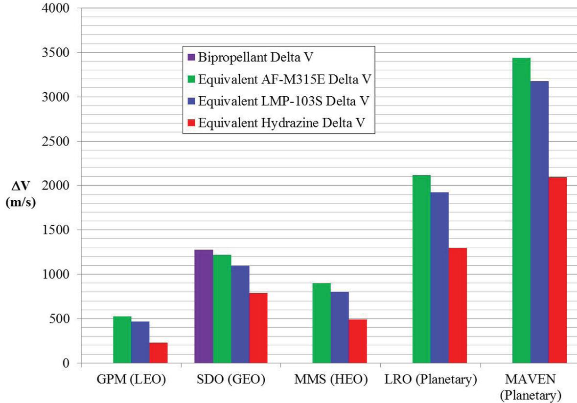
Figure 4  $\Delta V$  differences for the same propellant masses.
