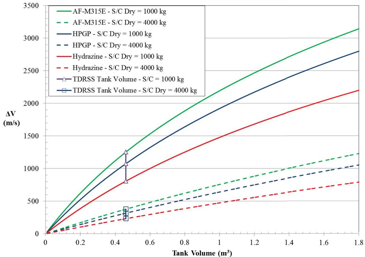
Figure 6  $\Delta V$  vs propellant volume for a generic spacecraft and tank.
