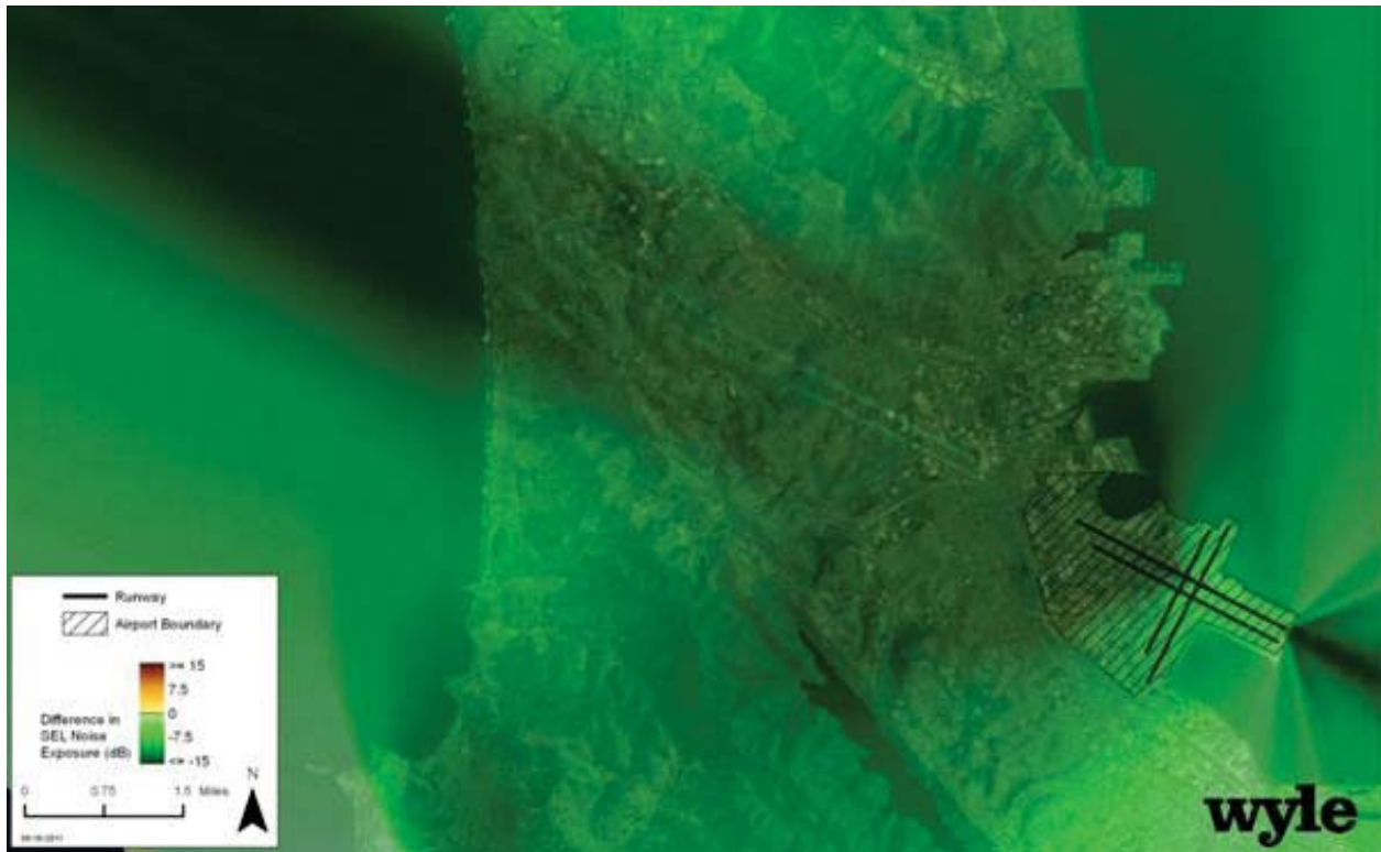
Figure 33 Difference SEL gradient comparing 2025 Baseline Vehicle and PSC on Departure at SFO
