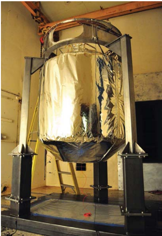
Figure 3: Vibro-Acoustic Test Article (VATA) being prepared in the MSFC acoustic test chamber for structural assessment of the thick MLI construction.
