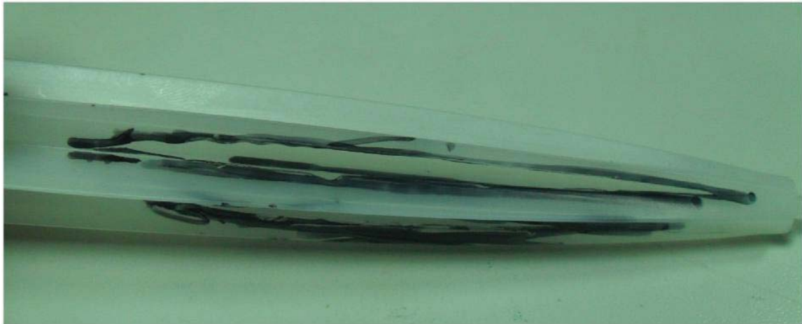
Figure 2. Initial spike samples with “short-shot” problems from Quick Parts
