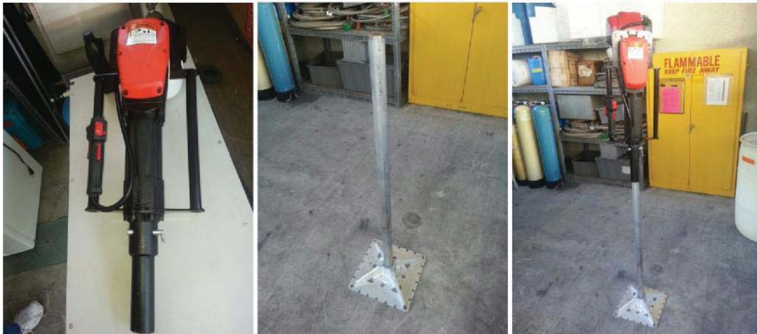
Figure 10: 4-stroke post-hole driver, driver-adapter, and assembled insertion system
