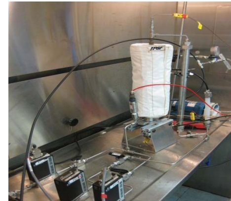
Thermal oxidation reactor at KSC
