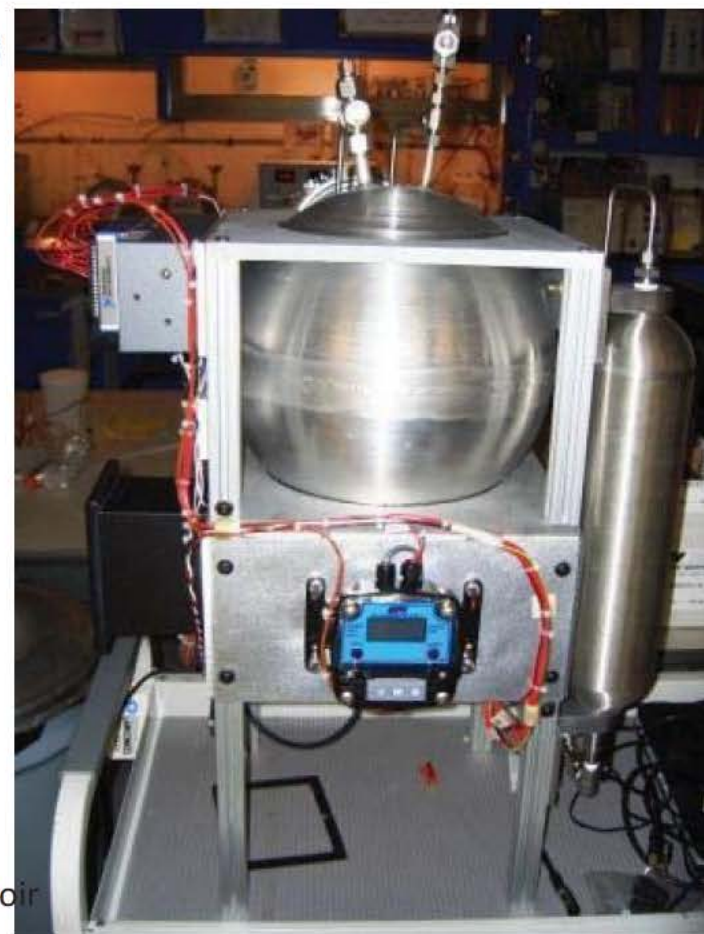
Membrane separator not included in the final version
