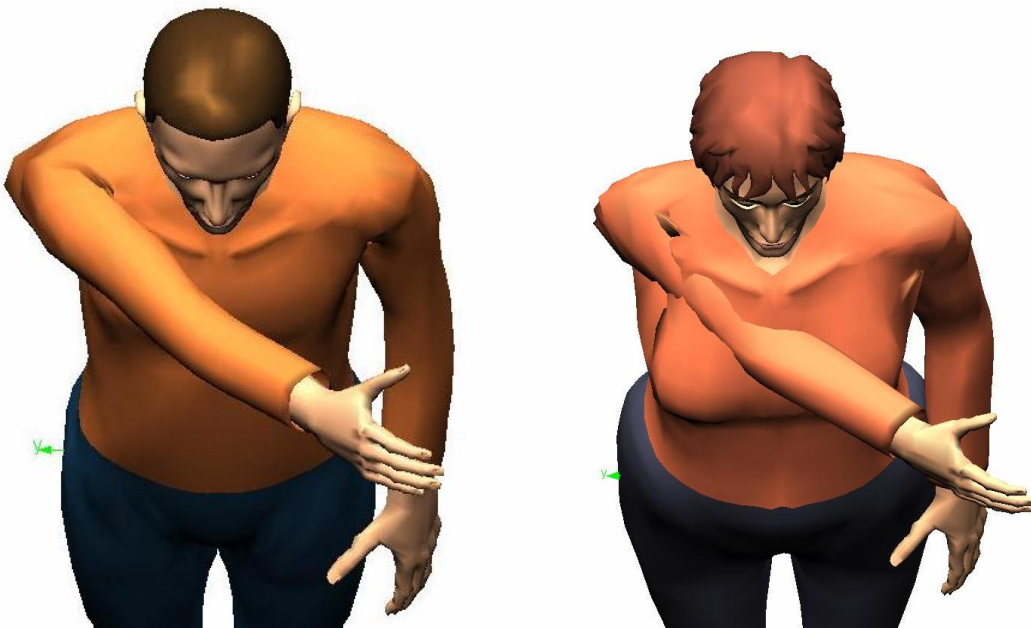
FIGURE 4.5.3.5.4-1 EXAMPLE OF SURFACE PENETRATION IN RAMSIS AS DEPENDENT ON SUBJECT ANTHROPOMETRY
