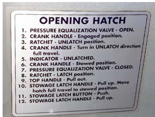
FIGURE 4.13.2.2.2.3-2 SAMPLE ISS HATCH OPENING INSTRUCTION LABEL
