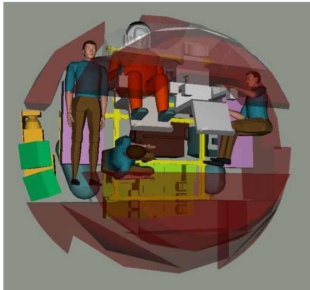
FIGURE 4.9.4.1-1 CAD MODEL SIMULATING 4 CREWMEMBERS PERFORMING POST-INSERTION CABIN RECONFIGURATION TASKS
