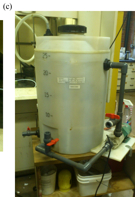
Figure 1. The PVDC-carbonization/CO 2 -activation tube-furnace system: (a) schematic representation; (b) the tube furnace and temperature controller; and (c) hydrogen-chloride scrubber.
