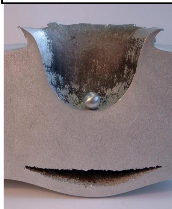
Comparison of size of projectile to size of impact crater
