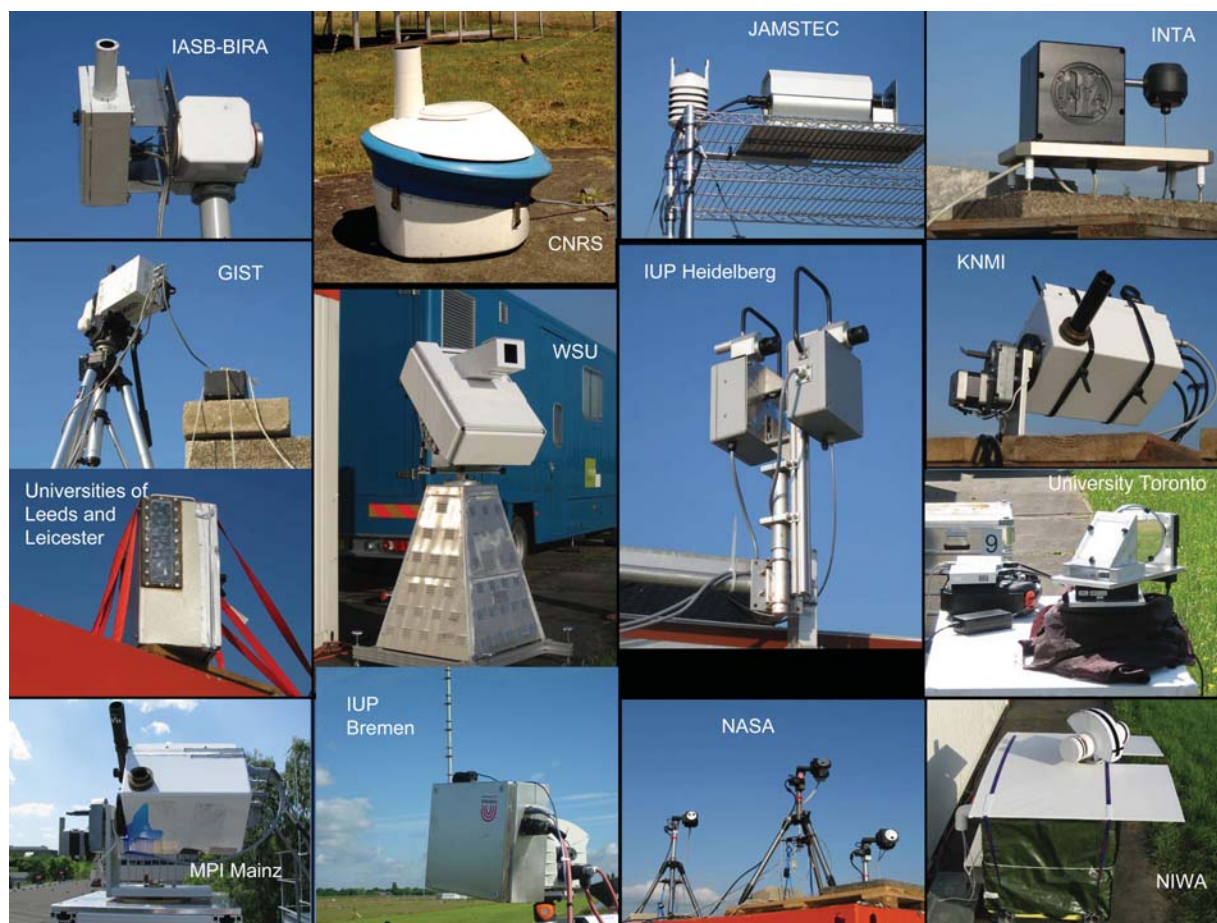
Fig. 3. Snapshots of the various optical instruments installed at the remote sensing site indicating the large variety of optical detection system designs actively involved in the campaign effort. Some images display complete stand-alone systems (e.g. WSU), others are only displaying the telescopes (e.g. NASA) that are connected to the spectrographs and detection systems by optical quartz fibres.
