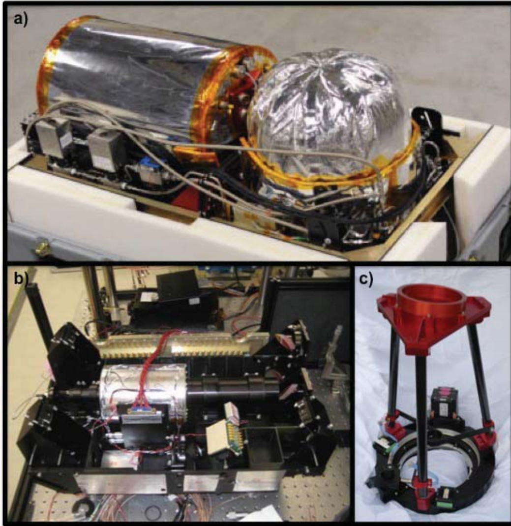
Figure 3. The fully assembled ACATS instrument (a) includes the receiver tube covered in insulation (left) and a pressurized telescope dome (right). A picture of the inside of the receiver subsystem (b) shows the etalon (silver device in the middle), the 24-channel array detector, and circle-to-point converter. The inside of the telescope subsystem (c) contains a motor to rotate the telescope and a HOE.
