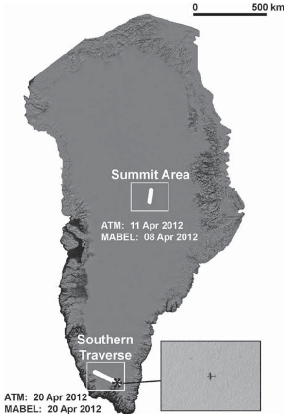
Fig. 2. Location map of the 50-km along-track Summit Area site and the 150-km along-track Southern Traverse site on the MODIS Mosaic of Greenland [17]. (Inset) Operation IceBridge P-3B captured in the NASA ER-2 Cirrus Digital Camera System [18] at the black “*”.
