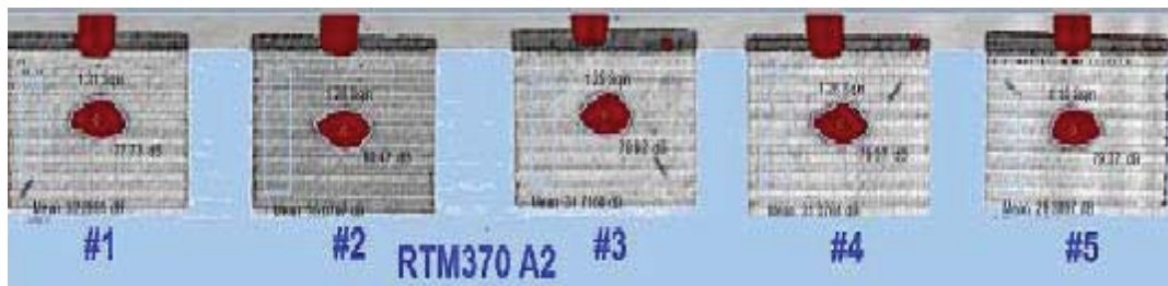
Figure 13. NDE Images of Impacted RTM370 Stitched Composites
