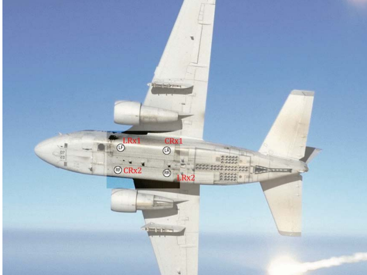
Figure 44. View of underside of S3-B aircraft used in flight tests of 11 June 2013. Antenna locations are LF, LR, RF, and RR, with corresponding connections to the two L-band and two C-band receivers (Rx1 and Rx2 for each band).
