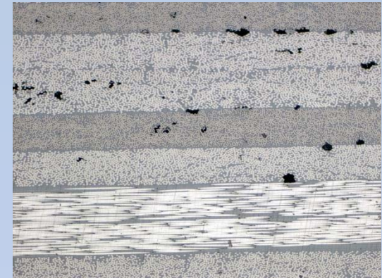
32-ply quasi isotropic panel, 100X
