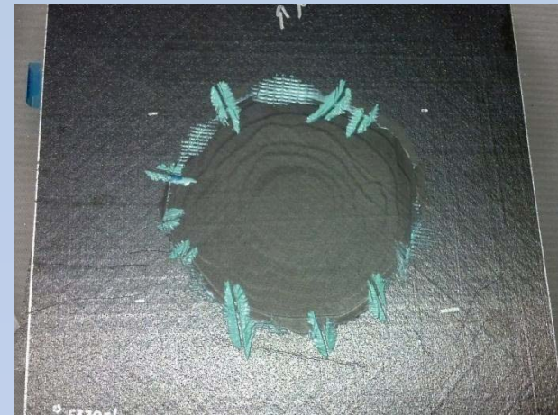
Panel B: Pre-cured Patch
