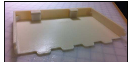
Figure B3: Half of the flat panel speaker frame after being 3D printed.
