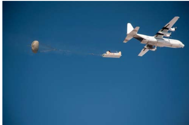
Figure 14b – DART C130 Release/Extraction
