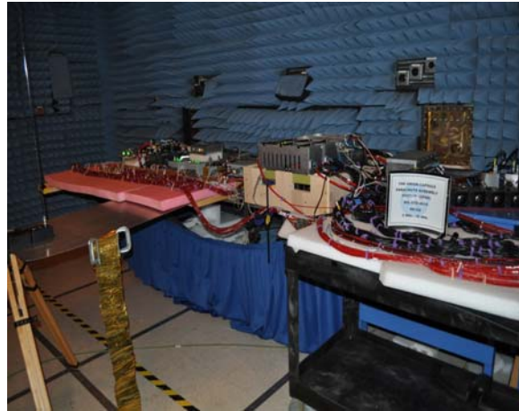
Figure 4a – CPAS Test Setup (2-30 MHz) Unshielded (VP)
