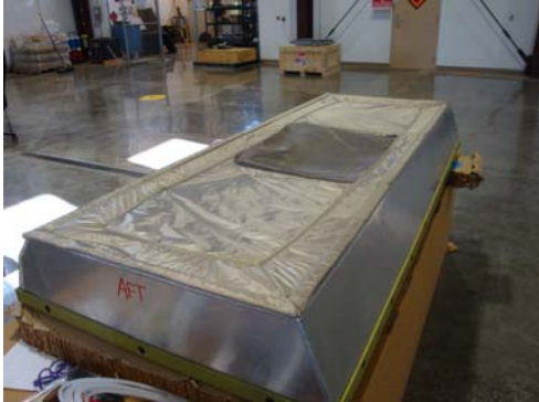
Figure 9 – Primary&Secondary Avionics Trays (Metal Sides, Conductive Cloth Cover, Mesh Window)
