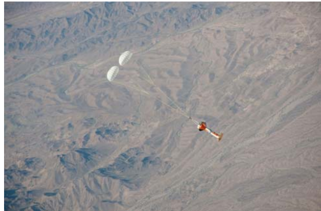
Figure 14c – DART Drop (2 Chutes out of 3 Simulating a 1 Chute Firing Failure)
