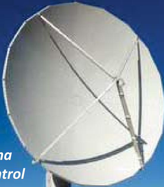
ASCS Canada 18-panel reflector and feed
