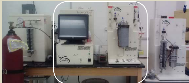
Figure 1. Helix system components. Only the center two components were used in the preliminary work which employed a stirred-batch process.
