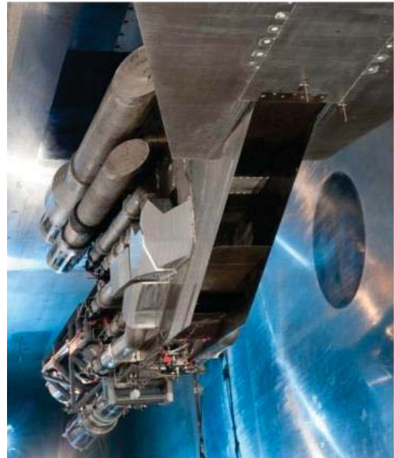
Figure 2. CCE LIMX installed in the NASA 10x10 SWT.
