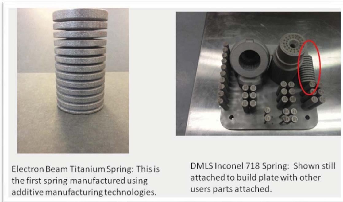
Figure 5 – Trial Spring Builds Showed Acceptable Build and Performance Goals were achieved.
