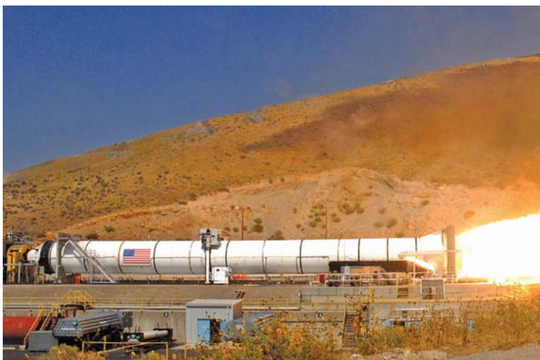
Fig. VII: SLS 5-segment Development Motor (DM-3) test firing
