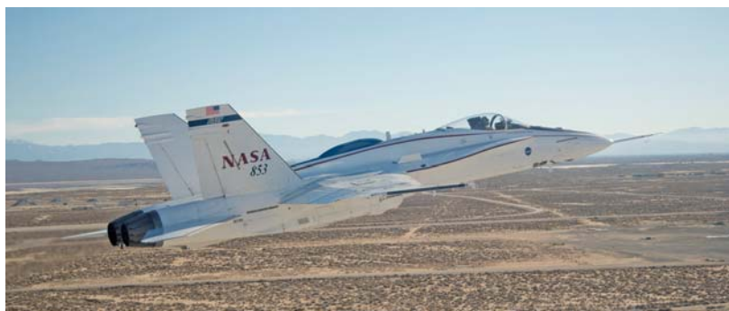
Fig. XII: SLS flight control testing using Dryden (DFAC) F/A-18 test plane
