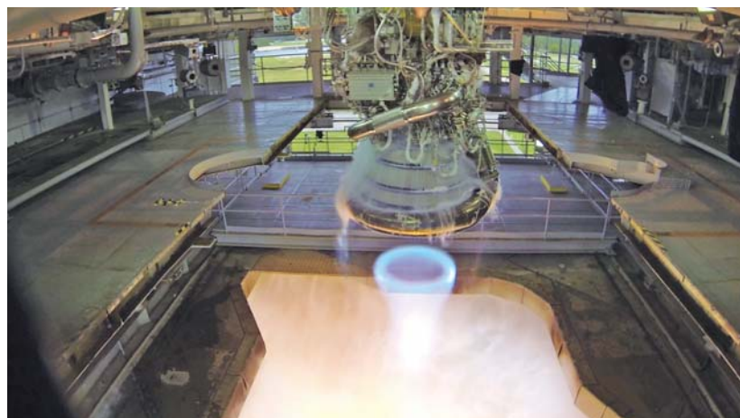
Fig.VI: J-2X engine test at SSC A-2 test stand
