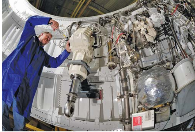
Fig. VIII: SLS booster aft skirt avionics/thrust vector control system
