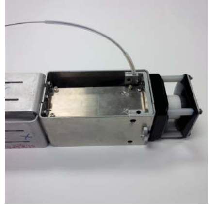
Fig. 5. Cable Guide with teflon tubes inserted.
