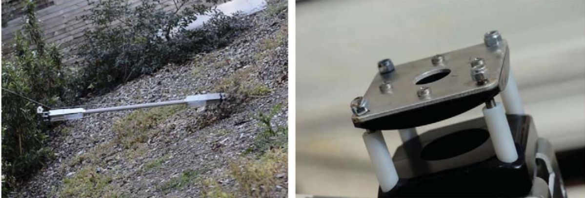
Fig. 16. Results of drop test. Left: End-cap and rod impact the ground. Right: Close-up of end-cap actuation area after impact, where the flanges on bottom spool cap have again sheared as the nylon spacers push through. Note that these forces are much greater than those expected under locomotion.
