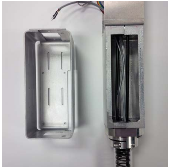
Fig. 7. Left: Redesigned battery compartment. Right: Original battery compartment.
