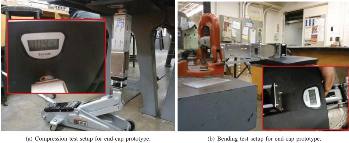
Fig. 14. Low-fidelity experimental test of prototype of modular end-cap assembly.
