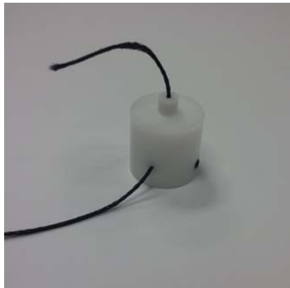
Fig. 10. Spindle with Vectran cable.
