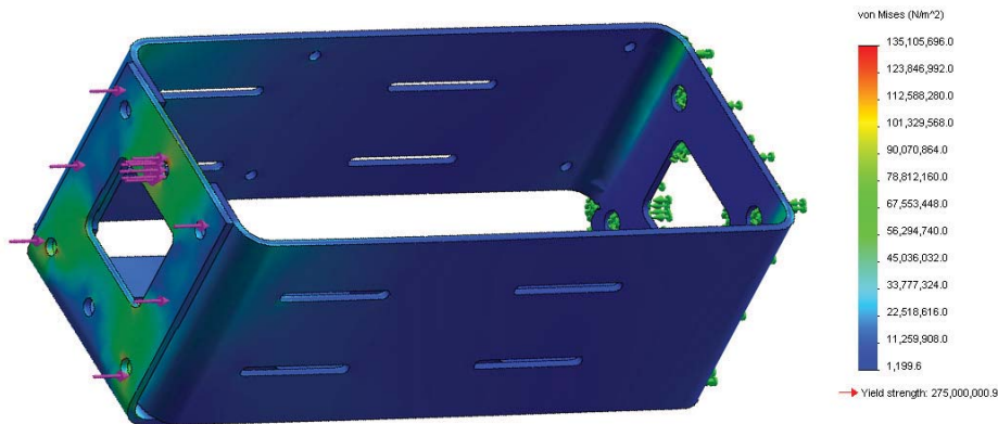
Fig. 12. FEA Test of the battery compartment.
