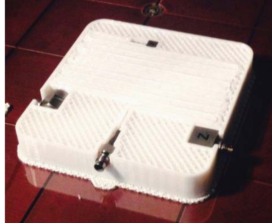
Figure 6. In-process images of sensor demonstration build. (a) Substrate printed up to component insertion point and sensors installed.
