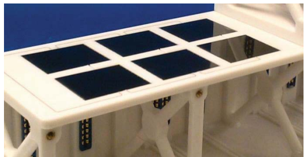
Figure 8(b). Completed 3U CubeSat prototype with embedded copper wire connecting a solar CIC array to the power bus.
