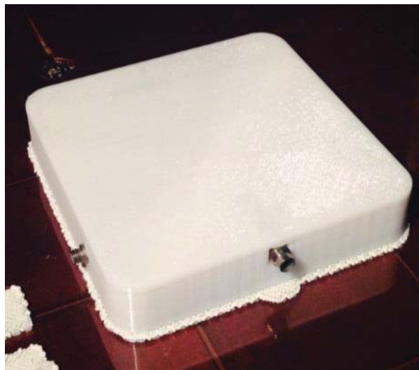
(c) Final layers printed above sensors to complete the piece.
