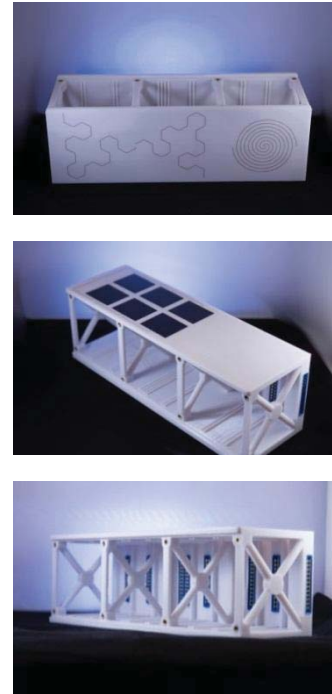
Figure 1. 3D-printed polymer 3U CubeSat.
