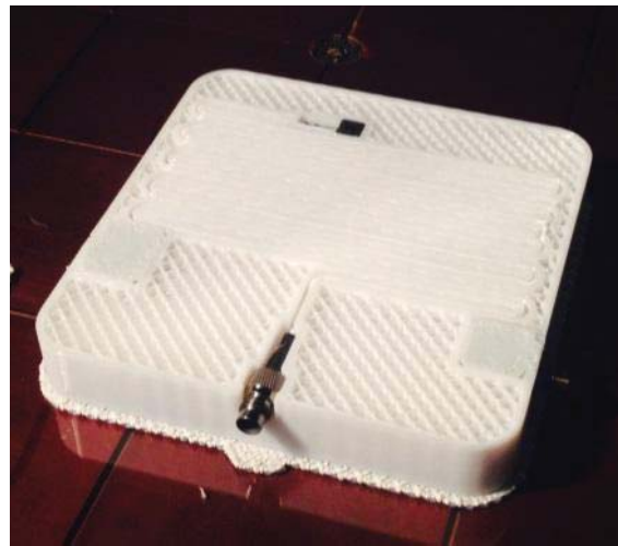
(b) 3D-printed caps installed above larger sensors.
