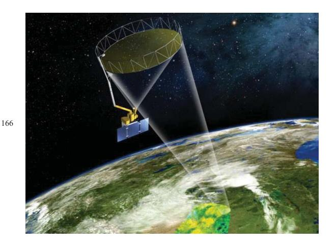
Figure 1. The SMAP L-band radar and radiometer share a common feed and reflector antenna system. The instruments conically scan across a wide swath allowing global
