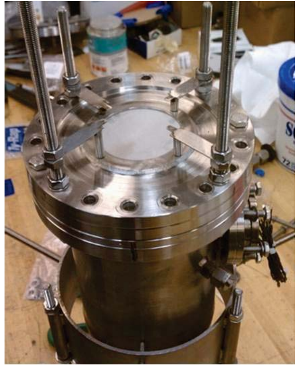
Figure 13.—Completed LAD Screen/Cup Assembly
