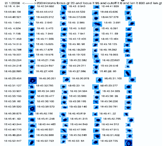
Figure 12: SPEC CPI images of ice particles in the lowermost stratosphere during CR-AVE.
