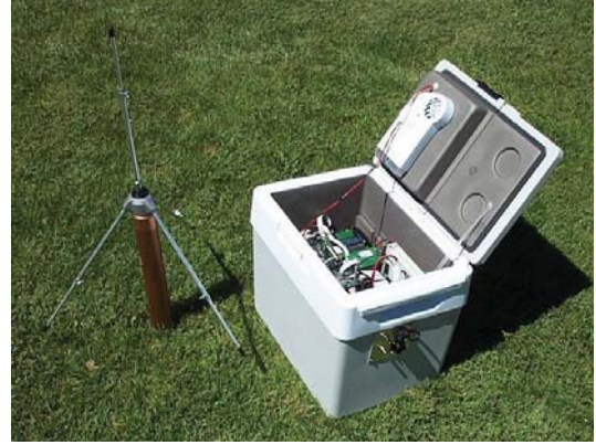
Figure 1. Portable LMA detection station
