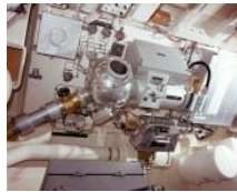
Skylab Materials Processing Facility Multipurpose Furnace System
