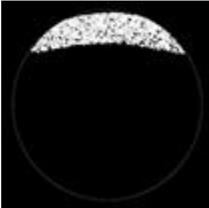
Pb-Sn alloy ( Sn in white ) Particles rise to top
