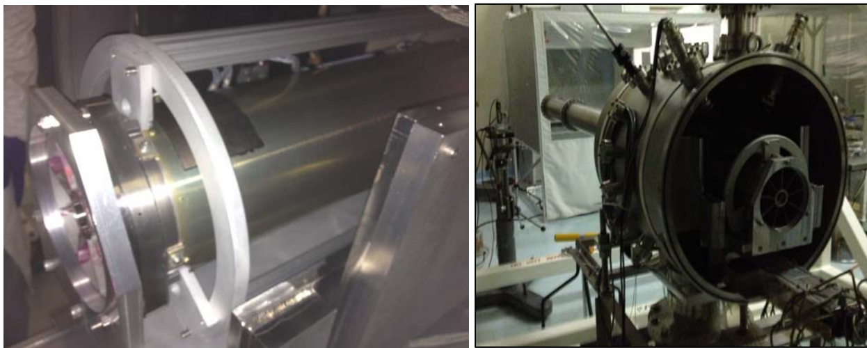
Figure 5. ART mirror module installed into a handling fixture (left) and inside of SLF bell housing for x-ray testing(right).
