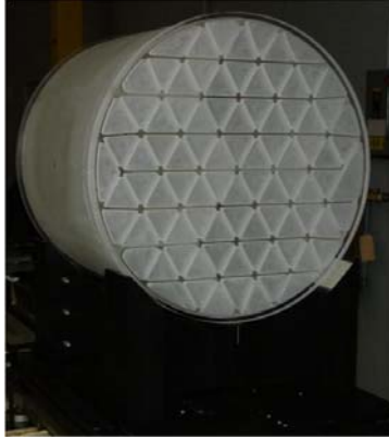
Figure 7 - A simple V-block mount was used to test the mirror horizontally during processing. This minimized the gravity effects during in-process testing.
