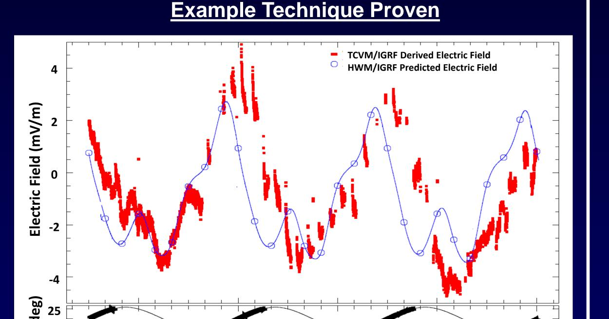
Measurement to enable Science Closure: A polar orbiting 1 km tethered cubesat would provide direct measurements of E||B to within 6 mV/m
