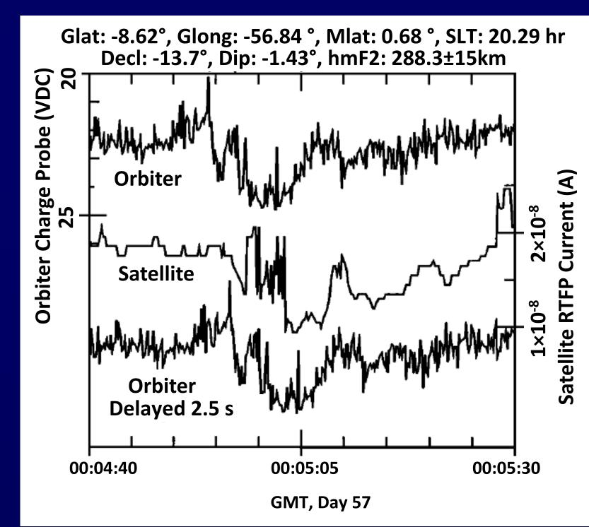
TSS-1R Orbiter data before and after a uniform time delay of 2.5 s is applied, thus aligning them with most of the prominent density structures at the satellite.
