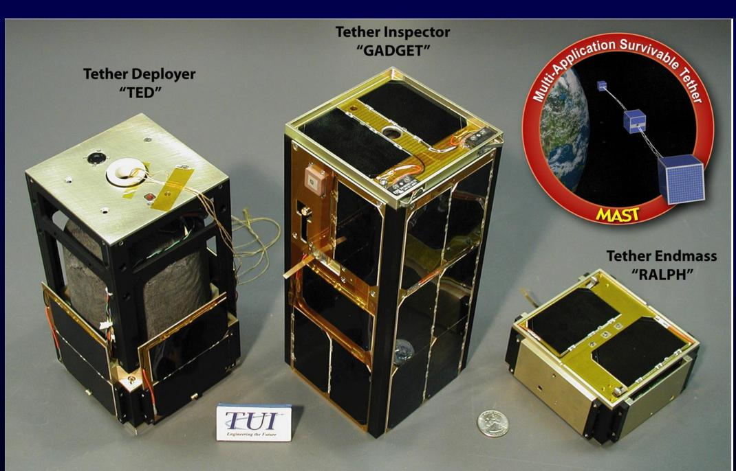
Tethers Unlimited (TUI) developed TRL7 CubeSat. Enables CubeSat with miniature
