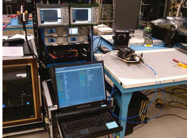
Figure 8 – Transponder Hardware Acceptance Configuration
