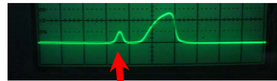
Pulse from failed cell.
