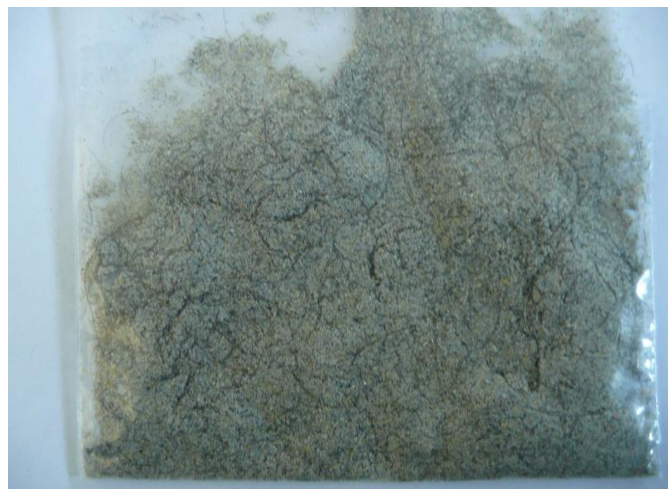
Figure 10. Debris that passed through the No. 35 standard test sieve. Mixed granular, fiber, and hair debris.
