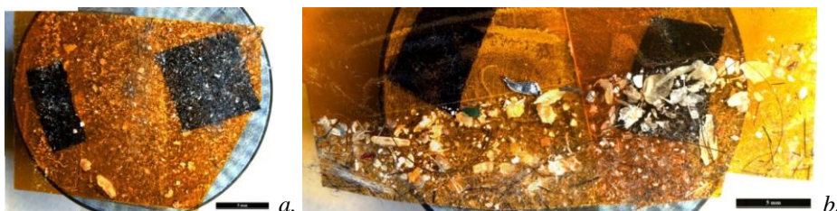
Figure 4. Cut sections of Kapton ® tape covering the vacuum HEPA filter element. Significant quantities of skin fragments, nail clippings, granular debris, hair, and fibrous debris are evident.
