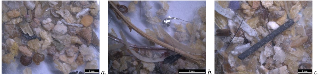
Figure 11. Granular debris retained on the No. 18 test sieve. a.) Typical debris showing dried skin and other unidentified debris at 10X magnification b.) a view showing a fruit stem and a large nail clipping at 8X magnification c.) a view showing a mechanical pencil lead fragment at 10X magnification.
