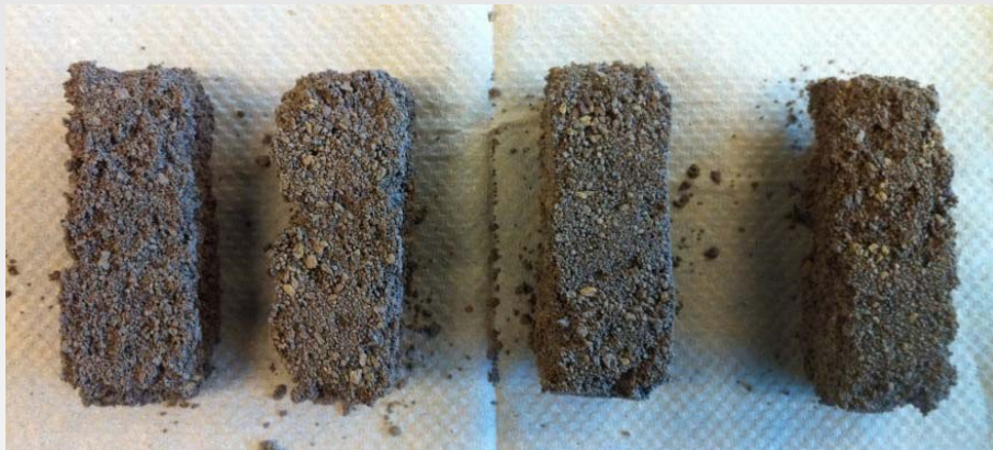
Sulfur-Bound bricks – Sublimation of sulfur resulted in insufficient content in bricks, bricks highly brittle
