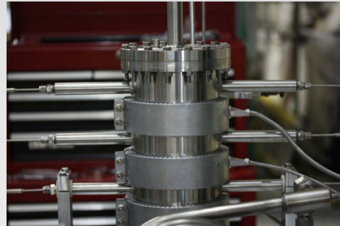
RWGS Reactor (with band heaters and thermocouples, no insulation)
