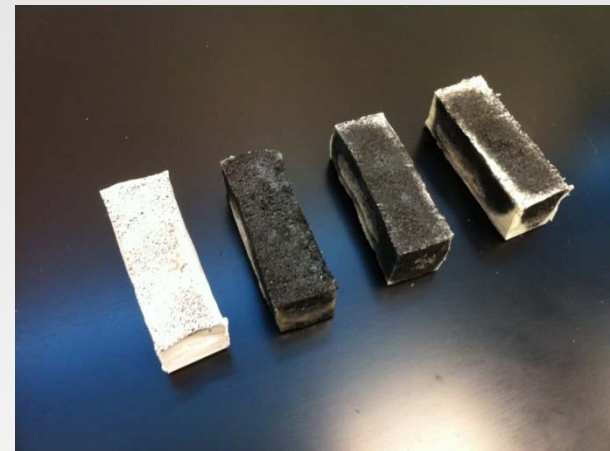
Polyethylene-Bound bricks – Repeatable method, uniform bricks, not entirely homogenous
