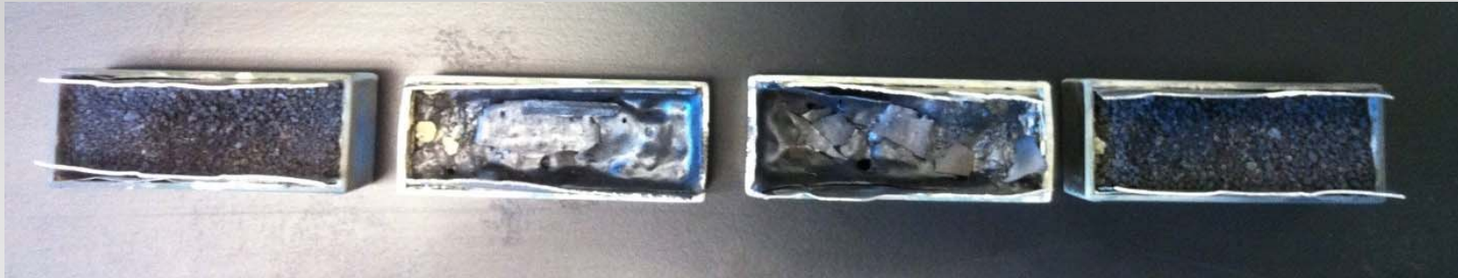
Sintered bricks – repeatability concerns (outer bricks not heated enough, center bricks heated too much within the same furnace)
