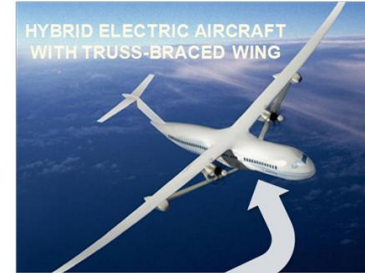
Gas turbine-battery hybrid
