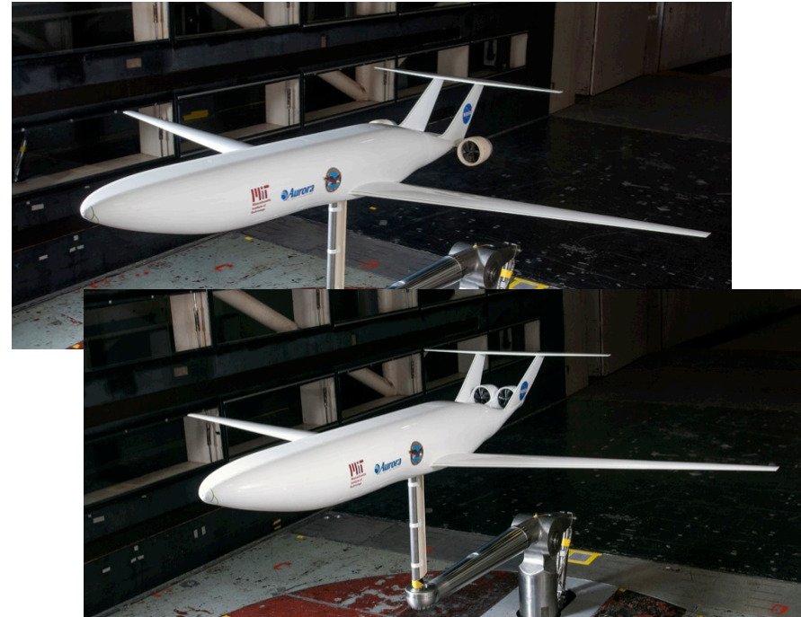
Direct comparison of podded and integrated configurations
