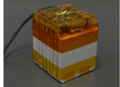
Figure 9. EM battery for testing.
