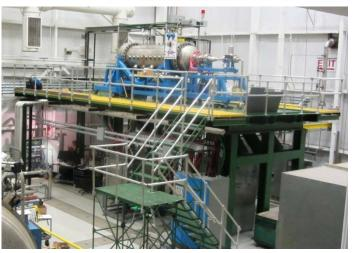
New Cooling Water System now provides 2 separate systems that cool induction coil and power feedthrough, induction heater and H<sub>2</sub>N<sub>2</sub> mixer respectively
