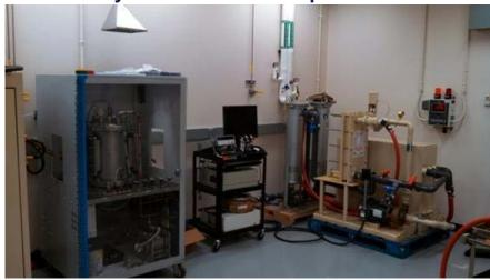
Completed CFEET system. Ready for W-UO2 and H2 testing
