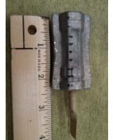
Above/Below: 7 channel WUO<sub>2</sub> fuel element post HIP and cross sections
