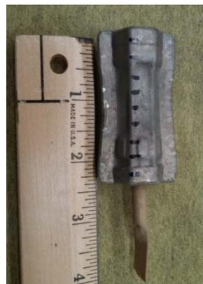
Above/Below: 7 channel W-VO<sub>2</sub> fuel element post HIP and cross sections
