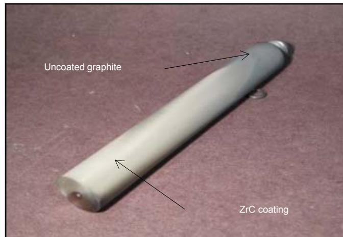
Above: Test Piece highlighting ZrC Coating
