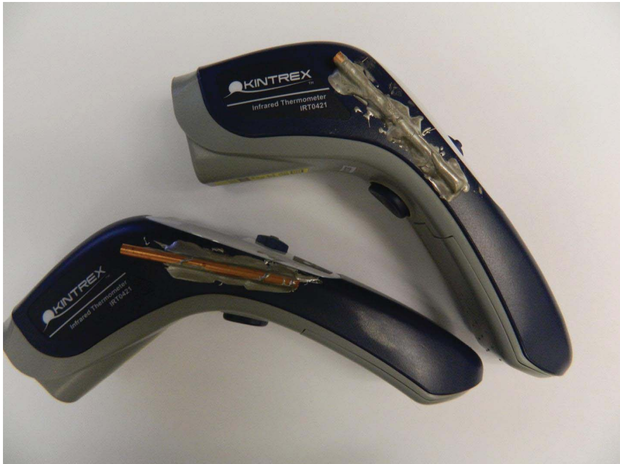
Figure 2.1-1. The IRTs used in this study with the thermal monitoring modifications.
