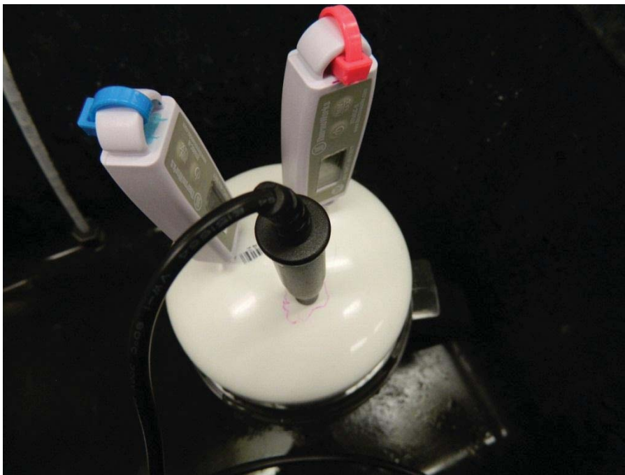
Figure 2.3.2-3. The assembled thermometer intercomparison bath.
