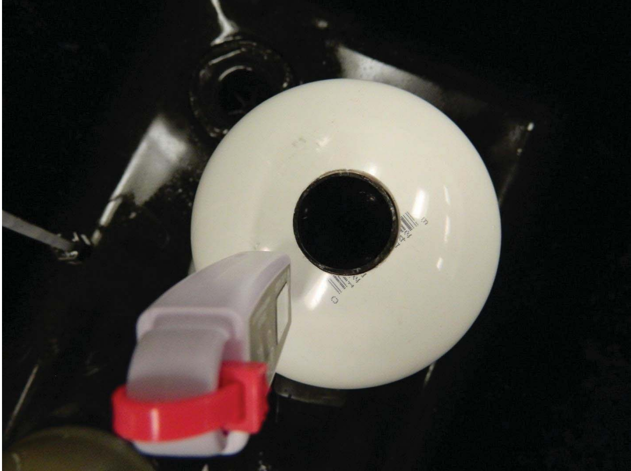
Figure 2.3.2-5. The IR “mini-cavity” in the constant temperature bath.
