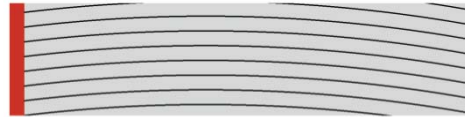
Figure 11. Steering path for the laminate with the highest flutter speed: core laminate = [-45^\circ / 45^\circ / 45^\circ]_s .
