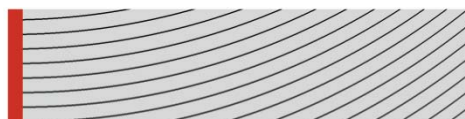
Figure 12. Steering path for the laminate with the highest strength: core laminate = [90^\circ / 90^\circ / 90^\circ]_s .
