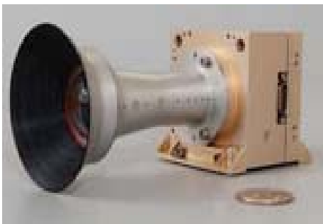
Figure 5. Picture of the ECAM camera under consideration for the NEA Scout spacecraft, shown with its baffle and electronics box. The ECAM uses the Aptina MT9P031 sensor that is certified for deep space.
