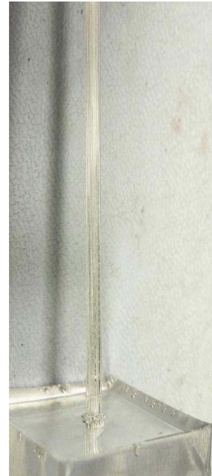
Capillary tube with ^6\text{Li} glass fibers in BC600 optical interface
