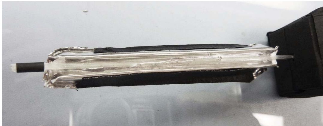
Capillary tube with ^6\text{Li} glass fibers submerged in BC600 optical cement and attached to PMT
