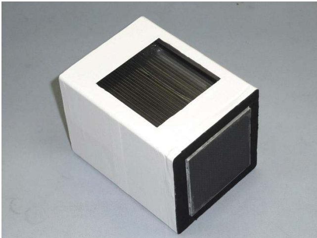
Wrapped in Tyvek, ready for PMT
