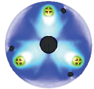
Figure 4. Finite Element Analysis View of End Cap Under Predicted Loads
