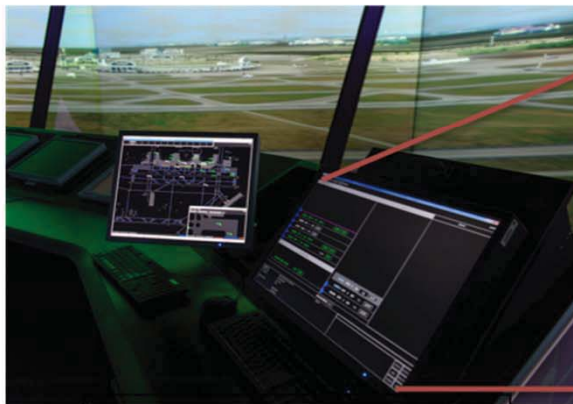
Local Controller Display
