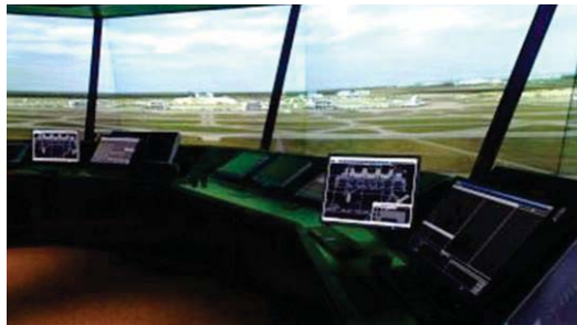
Figure 1. FFC tower cab simulator (Ground position on the left, and Local position on the right)
