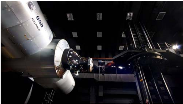
Figure 2: Full-size ISS mock-up (left) with sensor enclosure (center) mounted on the 6DOF robot (right), as seen from a ground perspective [1].
